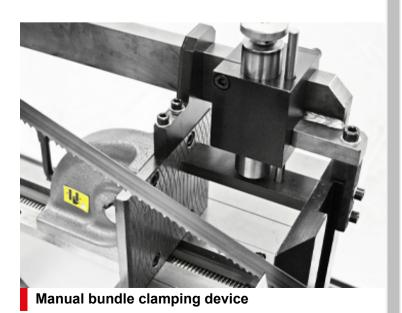
Device for clamping materials in layers and bundles with the use of an additional vertical clamping unit.
