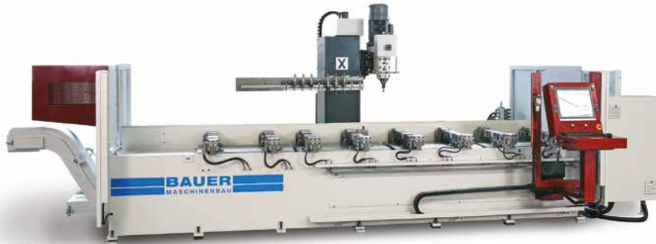
Bohrmax Z 40 with 8 hydraulic vices and pendulum operation
