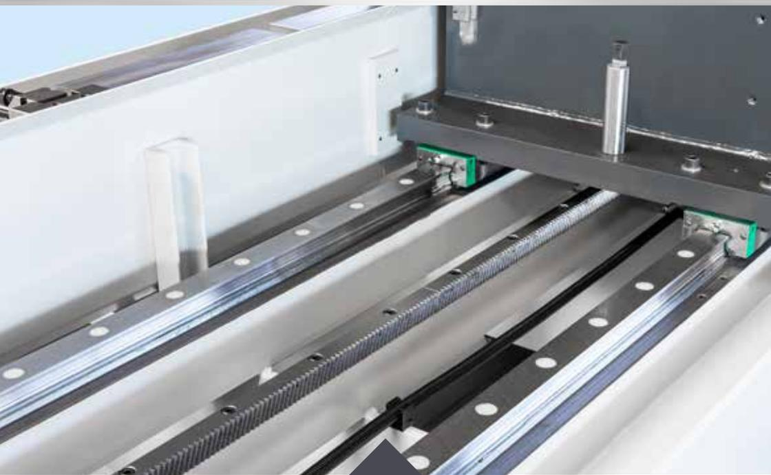
Largely dimensioned linear guides, large guide distance, feed x-axis through ground helical toothed rack, servo gear and servo motor.
