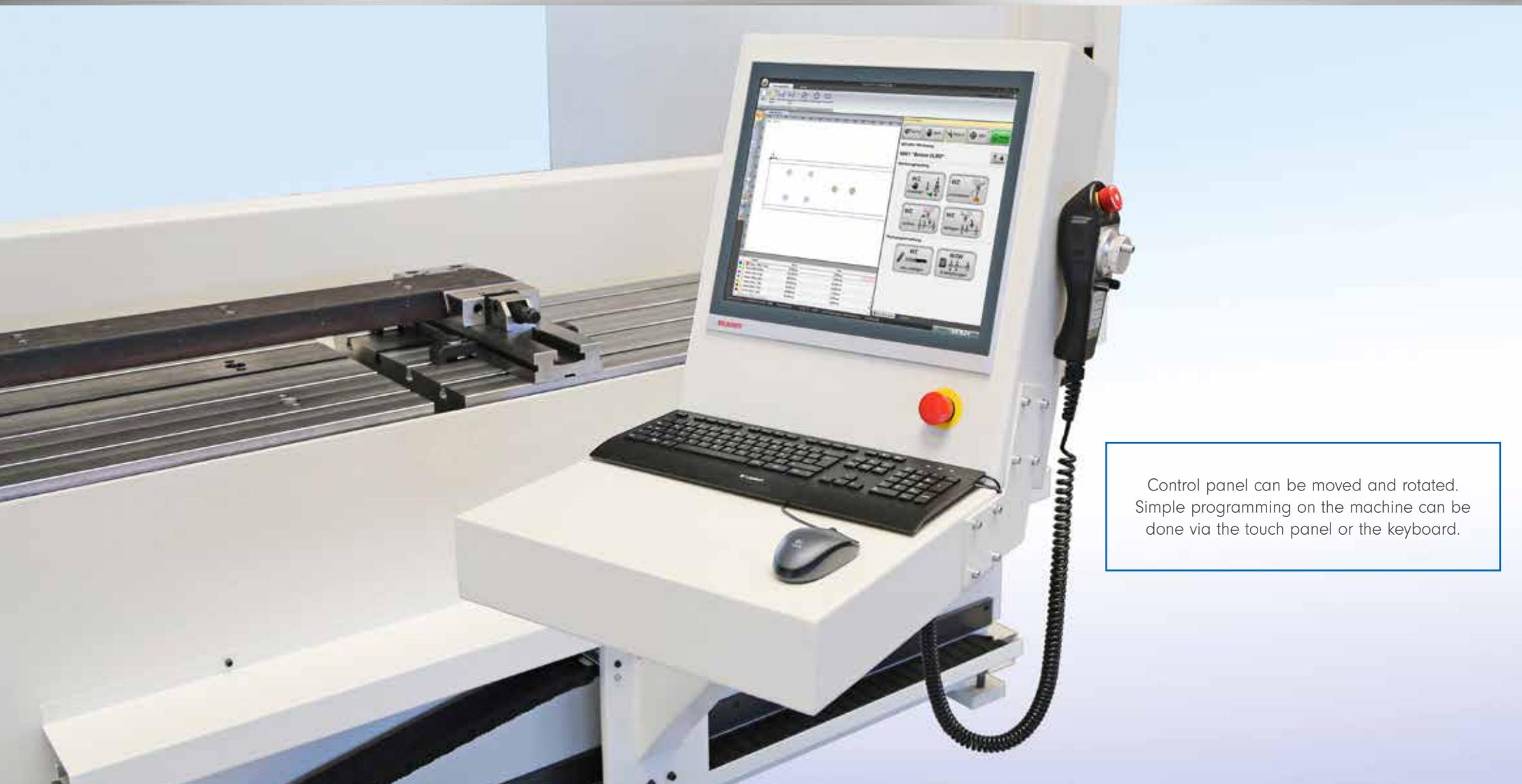
Control panel can be moved and rotated. Simple programming on the machine can be done via the touch panel or the keyboard.
