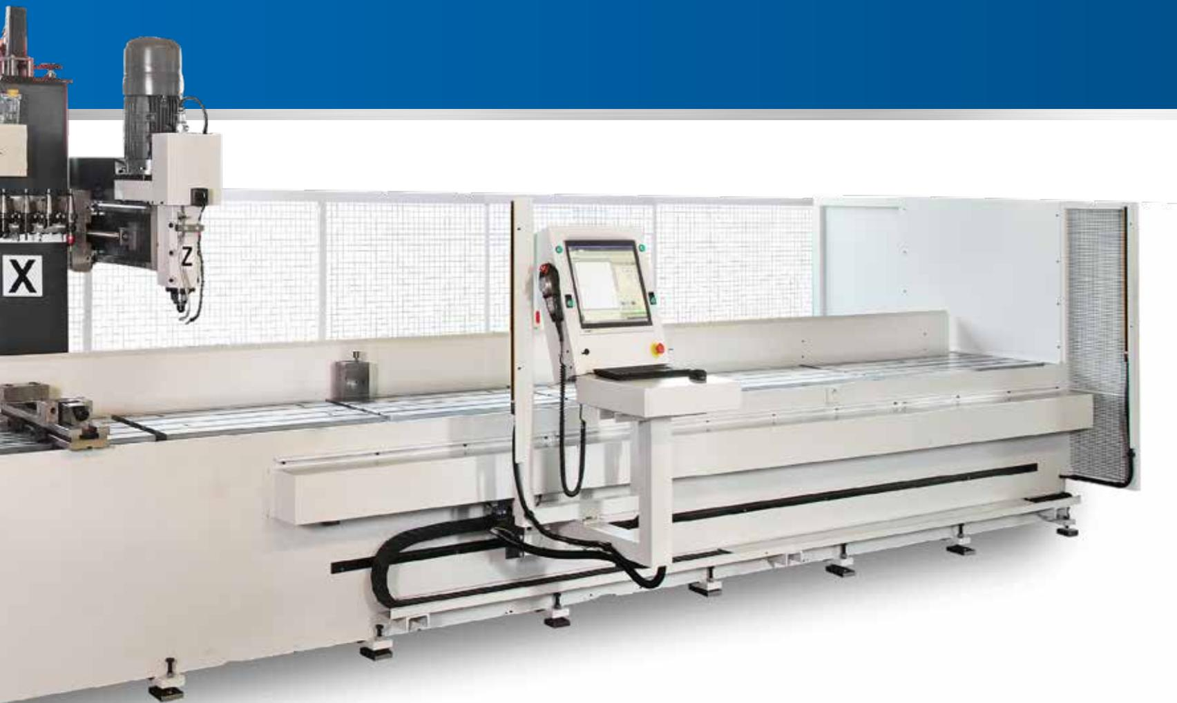
X axis 8050 mm, Y axis 580 mm, Z axis 700 mm, with option tool changer,
