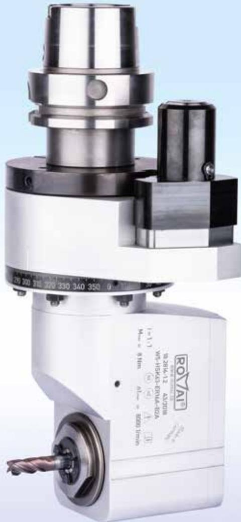
With the BOHRMAX, end faces can be milled or grooved with an angle head.
