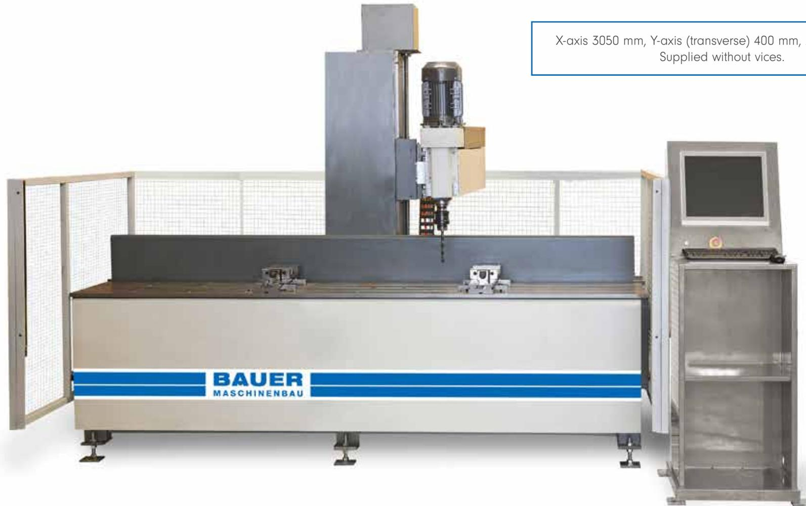
X-axis 3050 mm, Y-axis (transverse) 400 mm, Z-axis 400 mm.
