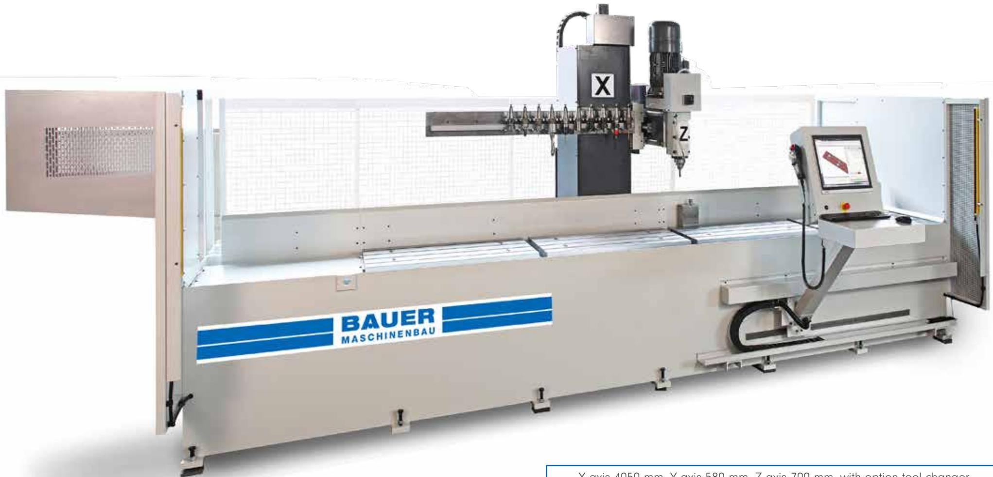
X axis 4050 mm, Y axis 580 mm, Z axis 700 mm, with option tool changer, gear 7.5 kW, tool holder SK 40, tool length measurement and manual control unit
