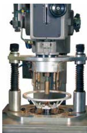
Multi-spindle headstock drilling detail of car handwheels.
