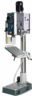
With rotating table plate and tilting support (MGI).
