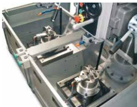
Hydraulic self-centering clamping tools for automation hinge.
