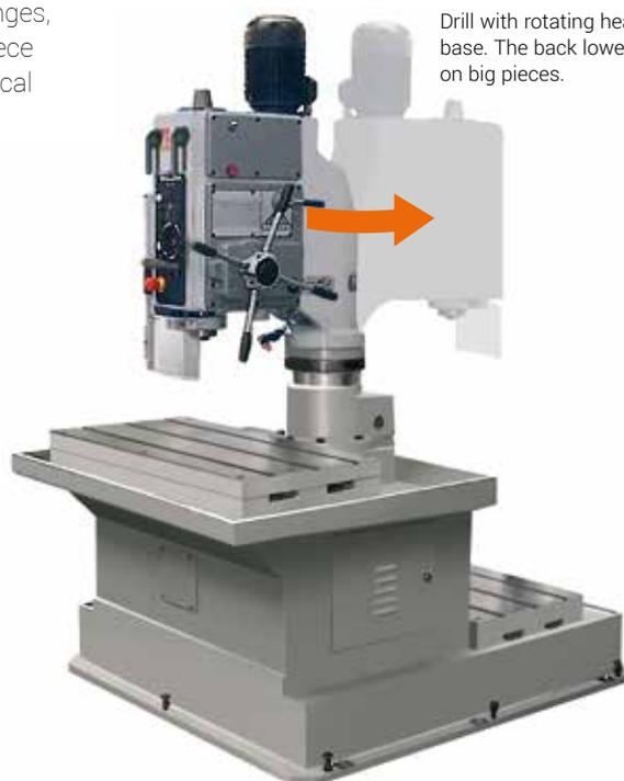
Drill with rotating head over double table base. The back lower table allows working on big pieces.
