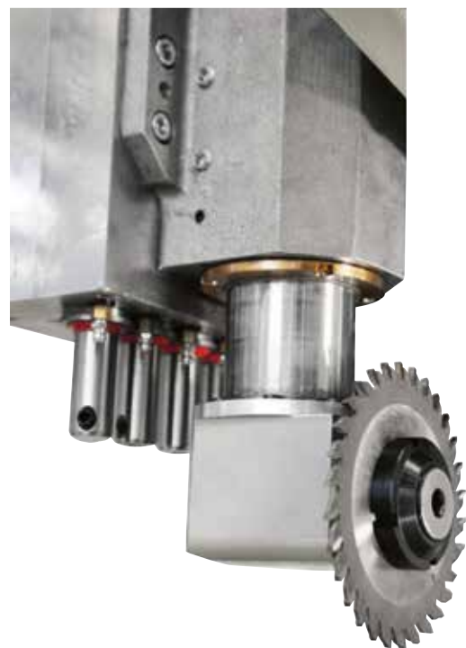
The 0°-90° blade assembly easily makes cuts or grooves in the X and Y directions.
