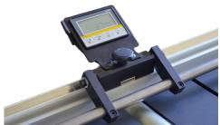
MRA has digital display for length showing instead band scale. MRA is fixed on steel rectangular bar guiding and the trolley was sliding on the well sliding segments.
