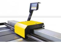
MDA has digital readout display for showing measuring length together MNCA is length stops with automatic position of required length. Part friendly to use device.
