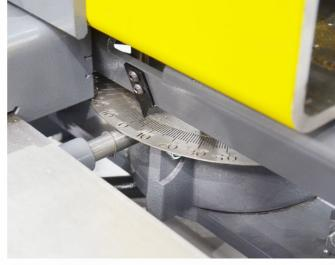
For maximum flexibility during angle cutting is Ergoline equipped by well seeable angle scale visible from operator place. The turning table has integrated cutting channel. This system ensures that during a angle cutting the saw arm with saw blade is always in the same position with cutting channel.
