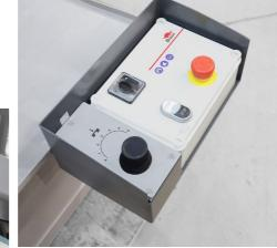
All control elements of the bandsaw are located on a simple understandable control panel, mounted on directly on machine pedestal at an optimal height for comfortable operation.
