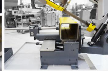
For material clamping, the bandsaw is equipped with a movable clamping vice that offers high flexibility. This vice can be easily moved to either the input or output side of the saw, allowing the operator to clamp material on the left or right side as needed. This feature is particularly beneficial for angular cuts, as it maximizes work efficiency and reduces handling times. Clamping of material ensure a fast clamp clamping system consisting of clamping handle with eccentric fixing lever.
