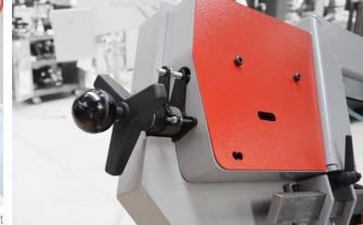
directly on the saw arm and right tension value is secure by electronic system to will not allow run a machine without correct tension or stop machine in the moment when saw blade is break.
