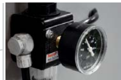
Input pressure indicator and regulation with a filter
