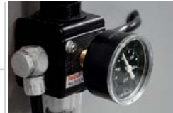
Input pressure indicator and regulation with a filter
