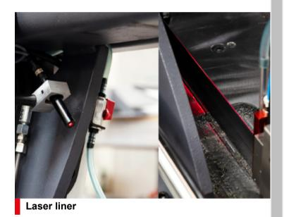
The laser unit copies the exact line in the saw band axis to the material. Laser Liner allows precise adjustment of the
