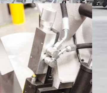
The saw blade guidance is enabled by ground horizontal elements of cemented carbide, always providing the greatest accuracy of the cut.
