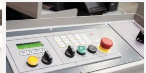
The central panel includes all of the control elements; it is located at an ergonomic height directly at the front of the machine.
