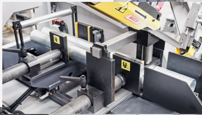
The saw blade guidance is enabled by ground horizontal elements of cemented carbide, always providing the greatest accuracy of the cut.
